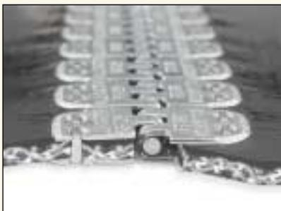
*Staples penetrate between carcass fibers without severing them. Staples are hammer-driven through the belt and then clinched crosswise to prevent belt tension from pulling against – and unclenching – the staples.*
