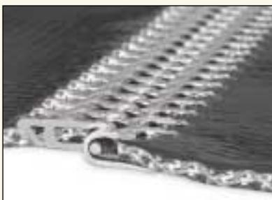
*Alligator® Lacing teeth enter parallel to the length of the belt and embed clear through the belt carcass. The design of the teeth ensures that once they are driven into the belt, the vital longitudinal carcass fibers are not severed.*
