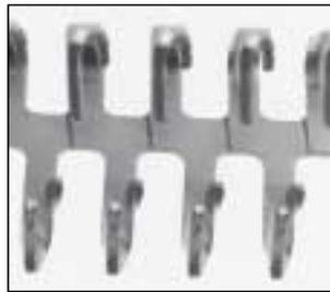
**Transmission belt lacing:** For flat power transmission belts up to 300 mm (12”) wide. Lacing is scored, so it can break away to fit belts narrower than packaged size.
