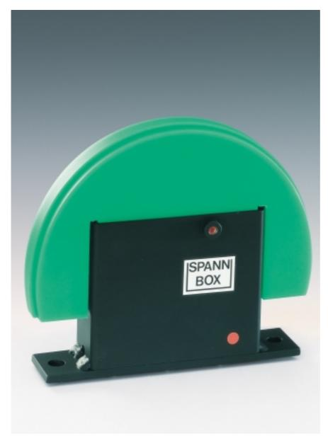
These chain tensioners are suitable for 180° chain returns. The radius of the standard size corresponds to a chain sprocket diameter of 140 or 200mm but can be increased on request. Fitted behind the drive, they allow chain stretch twice the length of spring travel to be kept under control.
