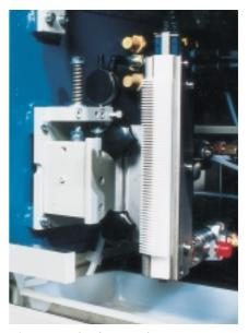
Glue spreader for wooden joints, made from Murytal® C natural
