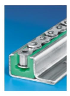
Thermoplastics subject to temperature fluctuations have a significantly higher coefficient of linear expansion than metals. That is why, for some applications, it is better for plastic guides to be held in place by a steel C-profile. (It also makes it easier and faster to replace them.)
