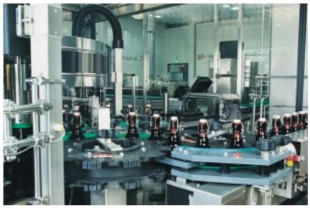
Bottling plant with discs, star wheels and worm screw made from Original Material "S"® black antistatic
