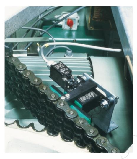
Incorporating mechanical limit switches or inductive proximity switches turns Murtfeldt's chain and belt tensioners into controllers capable of monitoring the smooth running of your production process. By activating a warning or triggering a machine shutdown in case of excessive chain/belt elongation or even rupture, they can help prevent serious damage.
