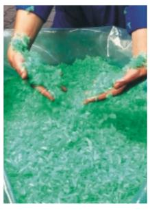
Material "S" 1000® is exclusively produced from ultra-macromolecular polyethylene. Its hi-tech manufacturing process mixes pure ultra-macromolecular polyethylene powder with ground Original Material "S"®. Under both high pressure and high temperature, this finely ground powder is then pressed into new semi-finished products. The result is a high-quality type of material impressive for its high abrasion resistance, good slide qualities and a very positive priceperformance ratio.
